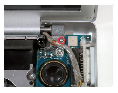
Remove the silver T6 Torx securing the ground loop in the display data cable to the casing.
