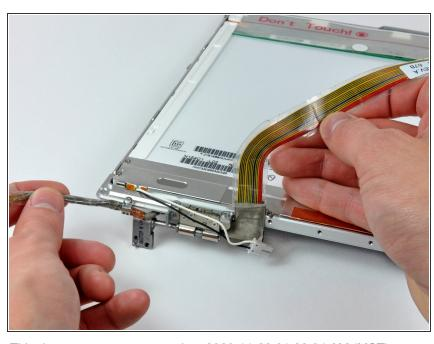
De-route the display data cable from around the right clutch hinge and remove it from the front bezel.
