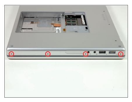
Rotate the computer 90 degrees again and remove the four 3.2 mm Phillips screws from the side of the computer.
