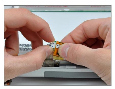
Disconnect the LCD backlight from the inverter by pulling its connector away from the inverter board.
