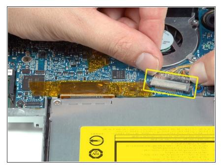
Disconnect the display data cable from the logic board by pulling sideways.
