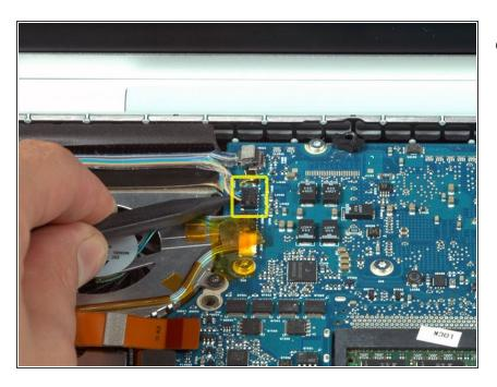
Disconnect the inverter cable from the logic board by placing a spudger beneath the cable and lifting up.
