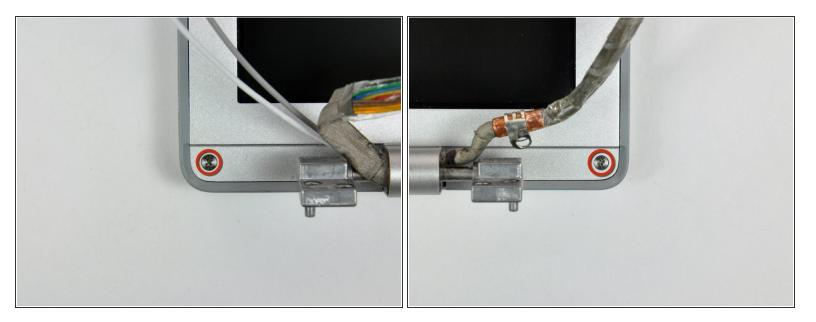
Remove the two 5 mm Phillips screws from the lower left and right corners of the display (two screws total).
