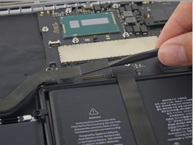
Use the flat end of a spudger to pop the I/O board connector straight up off its socket on the logic board.
