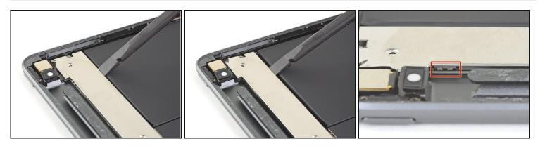
• Use a spudger to push the upper component bracket towards the upper edge and off of the clips located near the rear camera.
