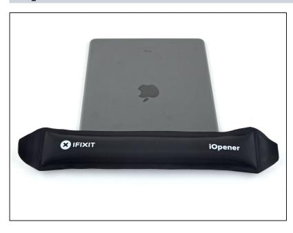
• Apply a heated iOpener to the top edge of the rear case for a minute.
