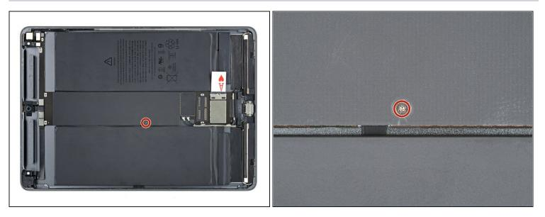
• Use a Phillips screwdriver to remove the 1.3 mm-long screw securing the logic board shield.
