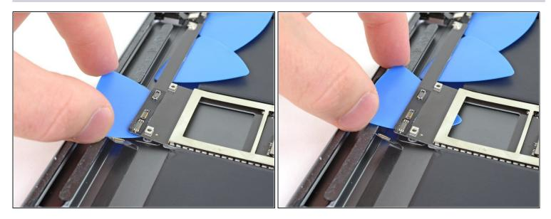
• Push the opening pick underneath the logic board to slice the adhesive.
