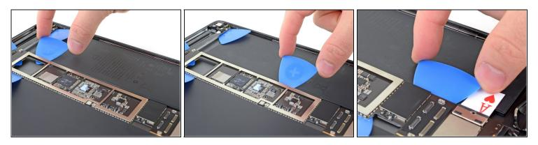
• Slide the opening pick down the right edge until you encounter the battery connector.
