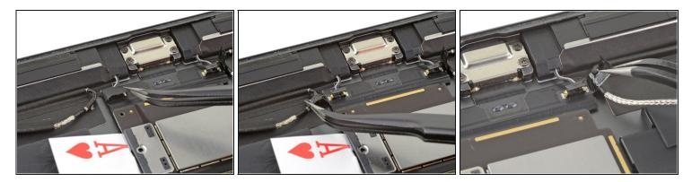
• Use a pair of tweezers to remove the tape from the back of both speaker connectors.
