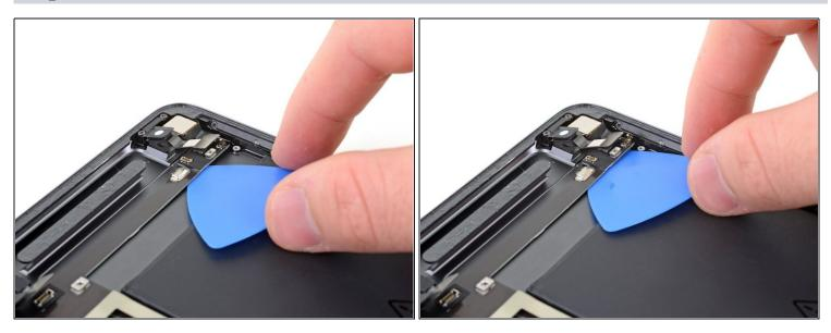
• Push the opening pick up towards the rear camera to slice the adhesive under the logic board arm.
