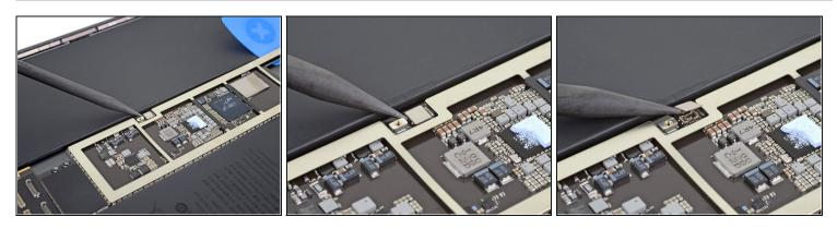
• Use the pointed end of a spudger to disconnect the Smart Connector cable by lifting straight up on the press connector.
