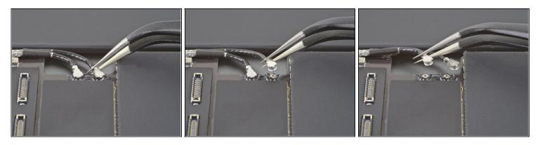
• Use a pair of tweezers to disconnect a logic board antenna cable by <u>lifting up on the</u> <u>cable as close to the connector as possible</u>.
