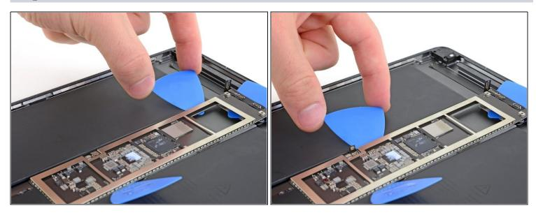
• Slide the opening pick down the left edge of the logic board until you get near the Smart Connector cable.
