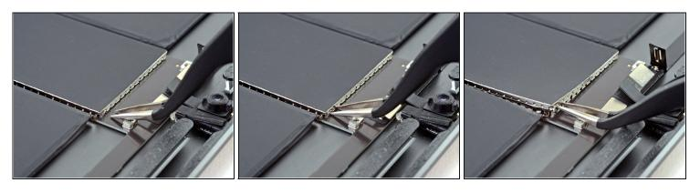
• Insert the tips of a pair of tweezers into the gaps under the the logic board shield on the upper right corner.
