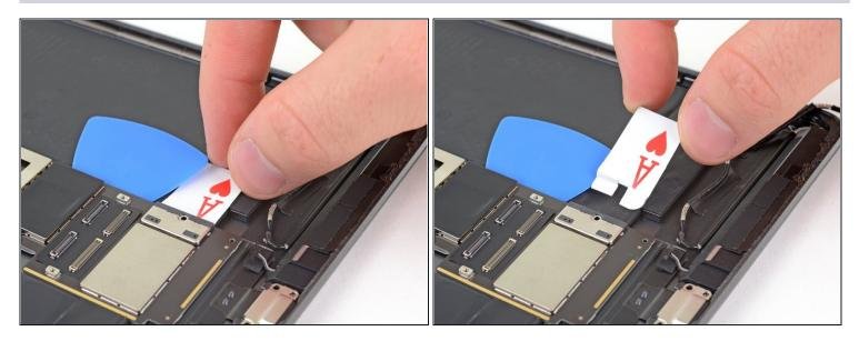
• Remove the battery blocker.
