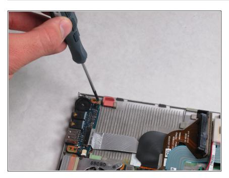
Remove the single 4 mm screw holding the port in place with the Phillips 00 screwdriver.
