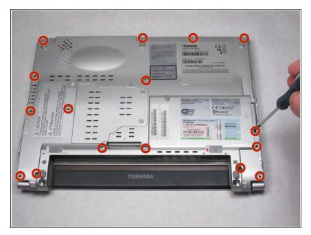
Remove the sixteen screws at the locations shown with the Phillips 00 screwdriver.
