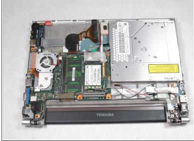
Pull up on the back casing and remove it, revealing the audio/usb port.
