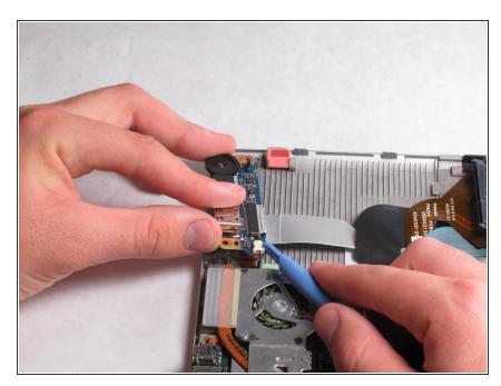
Use the plastic opening tool to disconnect the port from its power source on the laptop. This will be the wire connector with the white connection.
