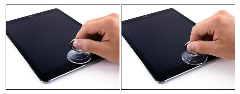
Place a suction cup over the iPad's front-facing camera and press down to create a seal.
