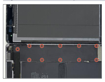
Use a Phillips screwdriver to remove the eleven 1.3 mm screws securing the EMI shield.
