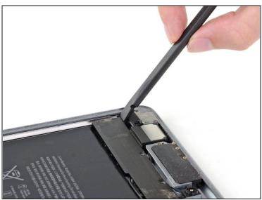
• Use the flat end of a spudger to push the left side of the upper speaker toward the battery just enough for the left speaker to slide out of its recess in the frame.
