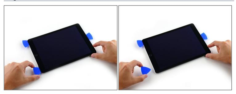
• Remove the right-hand opening pick at the bottom of the iPad.
