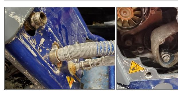
Connect bottom hose to pump hose without locking it in all the way. Pulling hard you will pull the top portion of the hose through and feed it all the way over to the right locked in place
