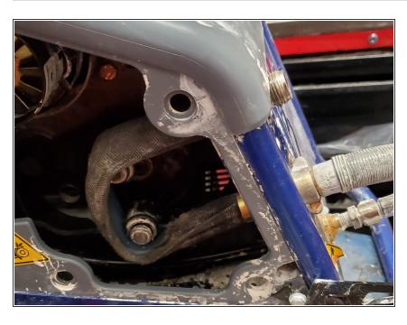
With the top hose attached make sure to feed around both ends of the pully and pull bottom hose through and push all the way to the right To reassemble your device, follow these instructions in reverse order.
