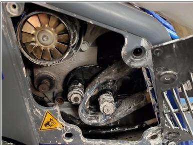
Remove 2 bolts holding the cover on
