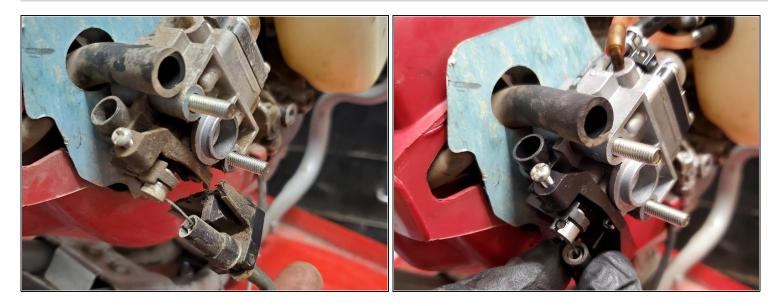
Remove old carburetor and install the new one. Remove the throttle cable and reinstall with needle nose pliers. Tighten throttle cable to carb part #16100-Z0Z-034
