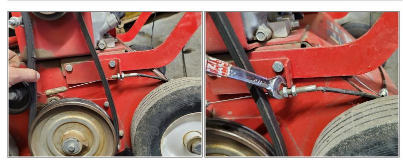
Remove old cable with needle nose pliers hook the new one on the same way. Tighten the new cable into place with the 10mm adjustment nuts at the bottom then reassemble the top portion
