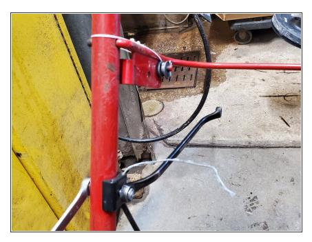
Remove one 7/16 standard nut securing cable
