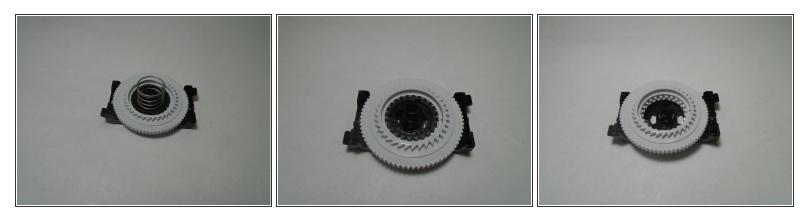
• Disassemble the adjuster assembly spring, small gear, large gear, and bracket in order to replace the broken component.
