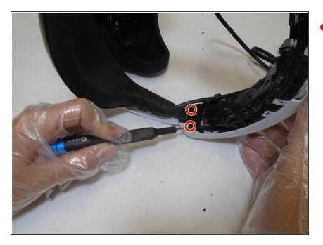
Remove a total of four 5 mm screws from inside the left and right sides of the headband using a Phillips #00 screwdriver.
