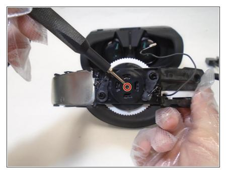
Remove the single 5 mm screw from the center of the headband adjuster using a Phillips #00 screwdriver.
