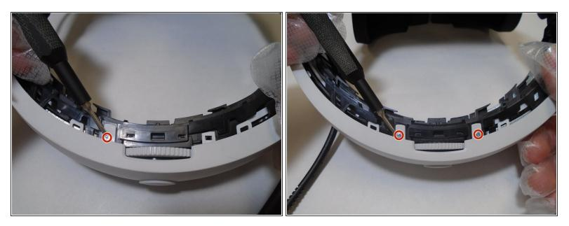
Remove three silver 5 mm screws that are securing the rear white cover of the band using a Phillips #00 screwdriver.
