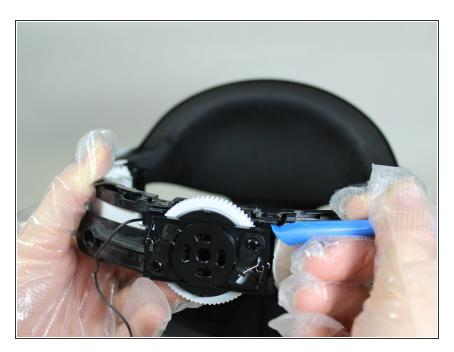
Gently pry the adjuster assembly away from the rear headband using an opening tool.
