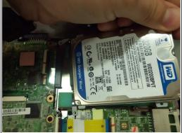
Remove the screws, and slide the hard drive free.
