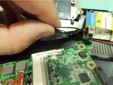
Remove the motherboard from the chassis, and disconnect a connector that is glued.
