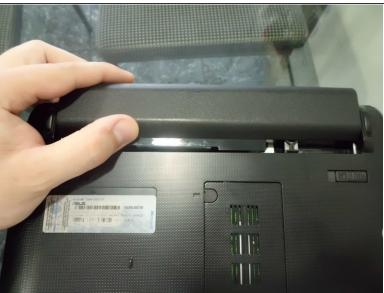
To remove the battery, unlock the marked tabs.
