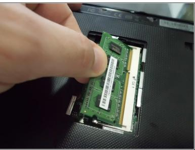
Lift the plastic cover and remove the SO-DIMM module.
