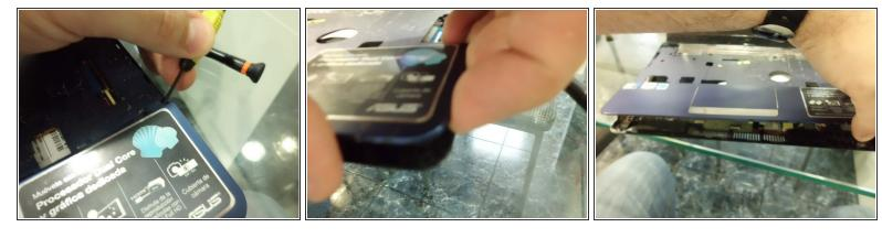
With a flat screwdriver, release two plastic tabs (1 on each side), and with pressure in the front, release the chassis.
