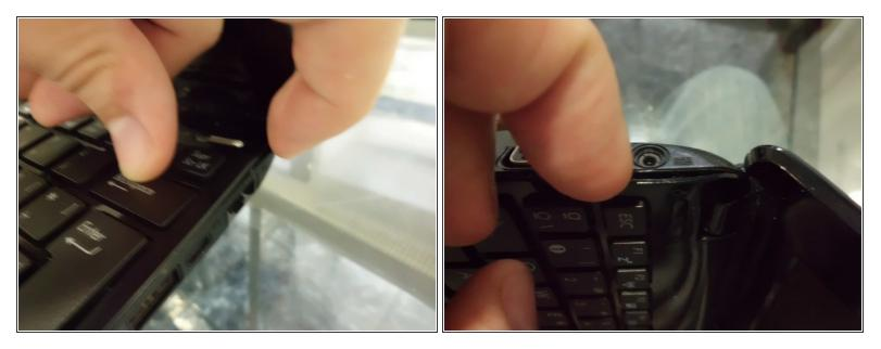
With an extraction tool, separate the keyboard chassis from the netbook, it has many tabs.
