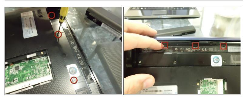
Unscrew 4 screws that are located in the battery compartment. Once removed, plastic tabs need to be removed on the upper part.
