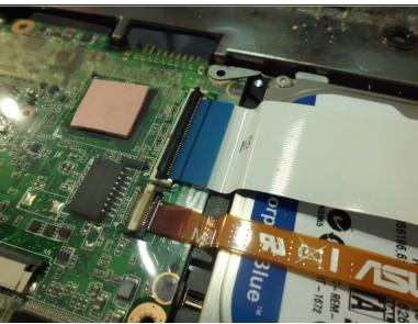
To disconnect the hard drive, two connectors need to be removed, pay attention to the connectors sides, the one on the left in marked as MB and the right is marked as IO.
