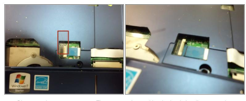
Disconnect the mouse connector. The connector has a white plastic tab that disconnects the connector.
