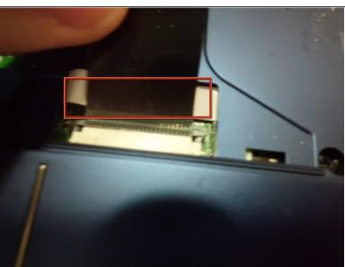
While separating the keyboard chassis, be careful with the keyboard connector. To remove it, simply slide the plastic retainer to be able to free it.
