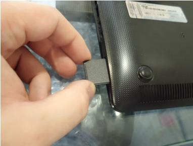
Remove the dummy SD-Card
