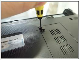
• To remove the memory, lift the plastic tab covering the memory screw with a small slot head screwdriver.
