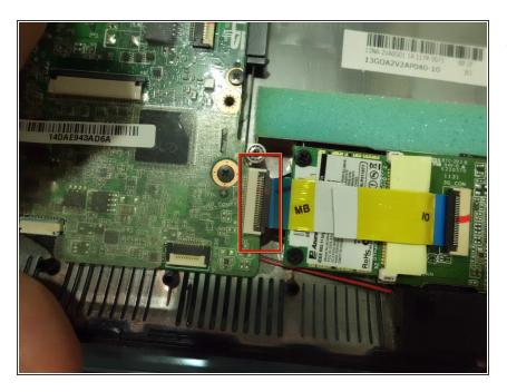
Disconnect the motherboard connector and the IO plate.
