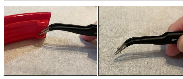
Remove the second hinge pin with precision tweezers and set it aside.
