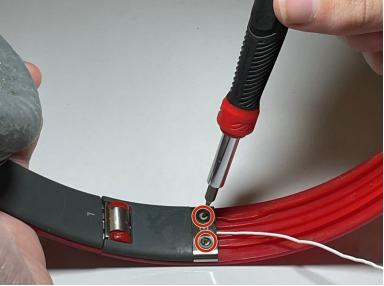
Screw both screws back into the metal brace.
