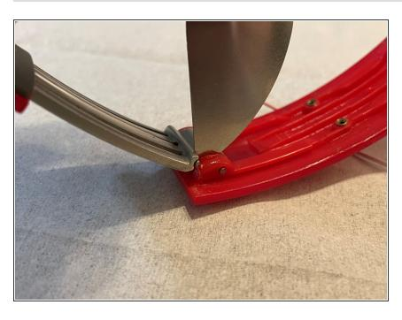
Slide the Jimmy between the metal earpiece and the plastic of the headband at the hinge.
