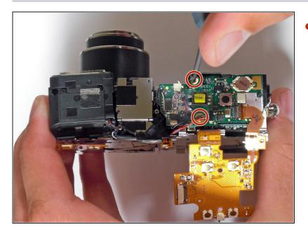
• With a Phillips #00 Screwdriver, unscrew the flash board.
