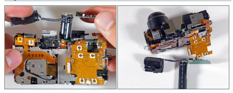
• Lift the entire three-part flash assembly from the camera.
