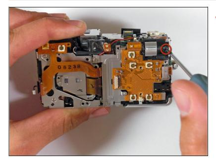
With a Phillips #00 Screwdriver, unscrew the zoom toggle switch and remove it from the camera.
