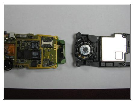
The black battery casing and logic board can now be separated for the following steps.
