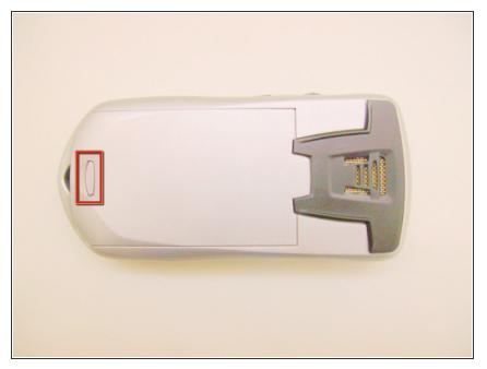
• With the back of the device facing you, press down on the button while sliding the battery casing away from the speaker to remove it.
