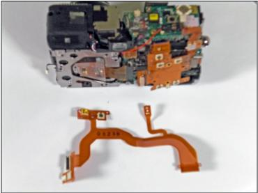
• Gently remove the entire ribbon cable connection to release the ribbon cable from the camera.
