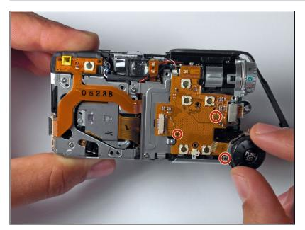
Be mindful of the pins as you lift up and remove the function/set button.
