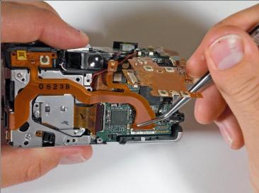
Lift the tab connecting the ribbon cable and detach.
