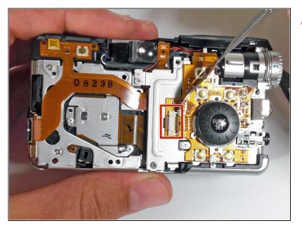
Gently pry up the tab with a metal spudger and remove the ribbon cable.
