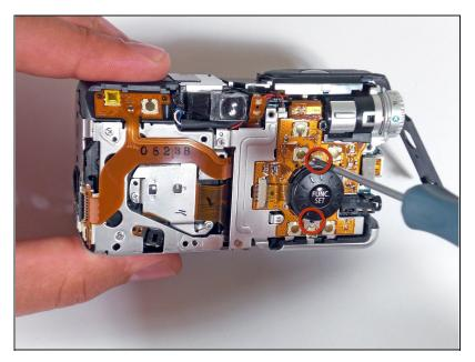
Remove the screws holding down the function set button.
