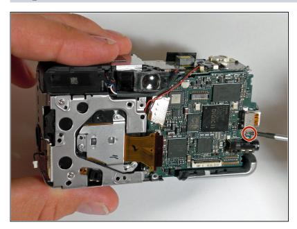
Remove the last screw holding the motherboard to the main body.
