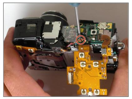
• Unscrew the circuit board from the flash unit.
