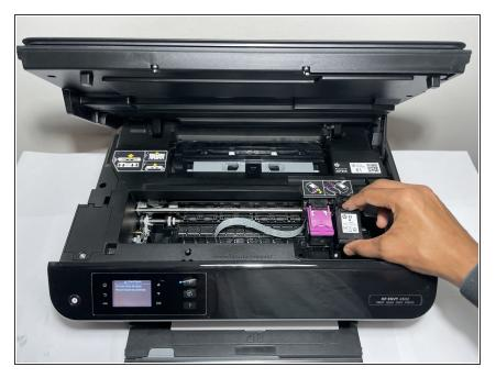
Once the body of the cartridge has completely dried, place it back into the slot in the printer.
