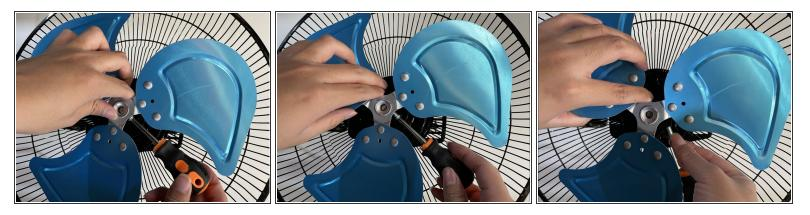
• Use the Phillips #2 screwdriver to remove the 1.4 mm screw that holds the fan blades to the fan.
