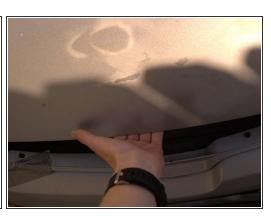
Reach underneath the front middle of the hood to open the hood.
