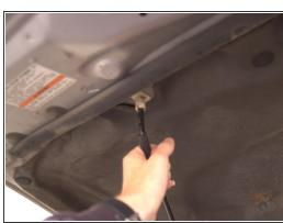
Once the hood is lifted, secure the hood by lifting up the hood prop.
