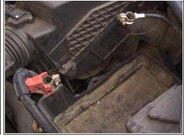
Once you have removed the mount, carefully lift the battery out of the vehicle.
