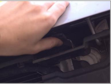
Press upwards on the lever on the underside of the hood in order to fully open the hood.
