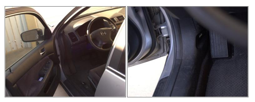
• Enter your vehicle from the driver's side, and locate the hood lever (in the footwell) near the far left side of the vehicle.
