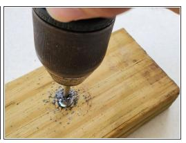
Place a center drill bit in the dent made in the previous step and start drilling until it expands enough to fit the standard drill bit inside it.
