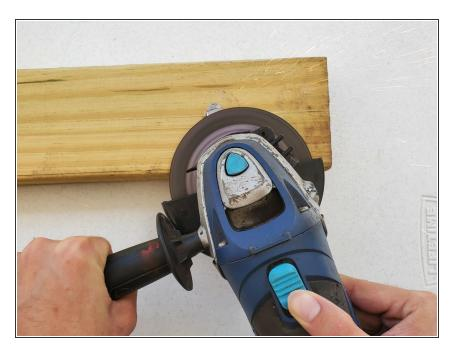
Use an angle grinder to grind the tip of the broken screw until its surface is smooth and even.
