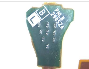
Close up view of the Top and Bottom side of the Touch Sensor PCB
