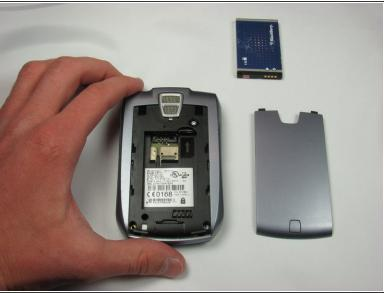
Using your fingernail, remove the battery by pulling on the notch on the top-right of the battery.
