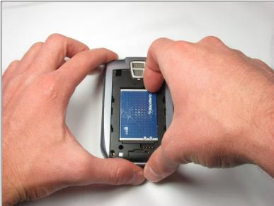
Replace the battery by positioning the top of the battery in the phone and snapping in the bottom.
