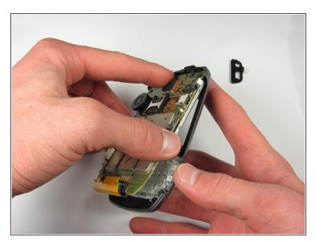
Replace the logic board by sliding it into the front cover.
