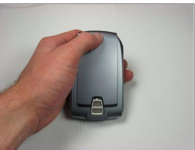
Replace the battery cover by sliding it against the device and snapping it into place.
