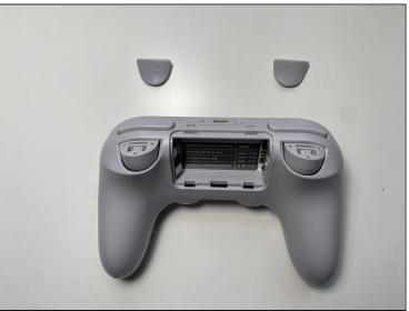
• Remove L2 and R2 trigger buttons by pushing them away from the grips.
