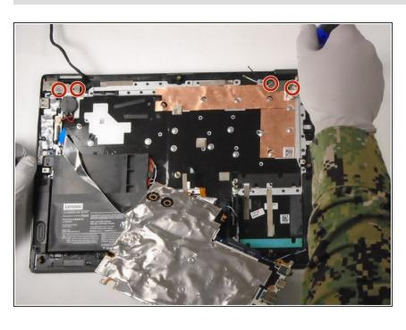
Use a Phillips #00 screwdriver to remove the four 5 mm screws from the left and right hinges (two screws on each hinge).
