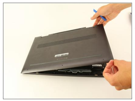
• Lift the back panel to remove it from the laptop.
