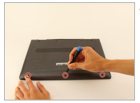
Use a Torx T5 screwdriver (T5 bit) to remove the three 5mm screws near the bottom edge of the laptop.
