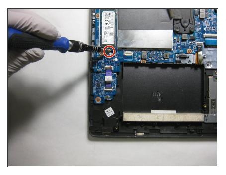
Use a Phillips #1 screwdriver to remove the single 4 mm screw securing the SSD.
