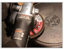
Grind off the black coating of the entire surface to expose the shiny bare metal.
