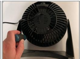
Remove the 6 screws from the backside of the fan.
