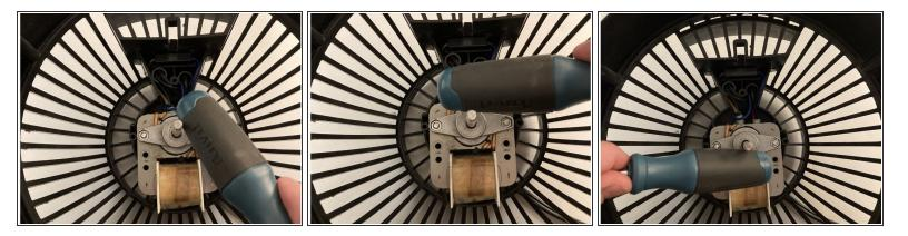
During reassembly, re-align the bearings by tapping on the shaft.
