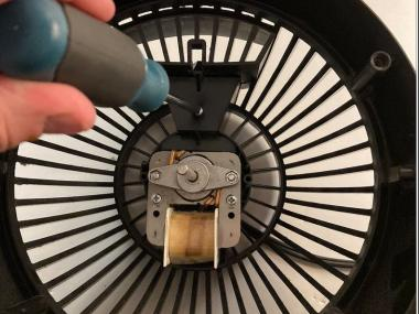
Remove 1 screw inside to detach the plastic wire covering.
