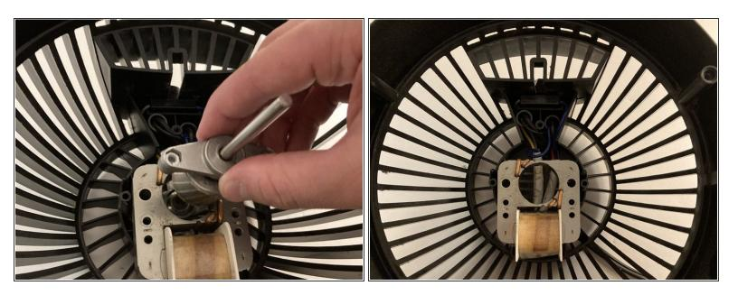
Remove the rotor and front bearings by pulling.
