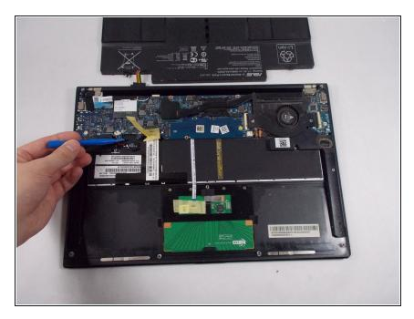
Remove the battery from the laptop by lifting it up and out.
