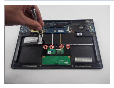
Use a Phillips #1 screwdriver to remove all four 6 mm screws from the trackpad.
