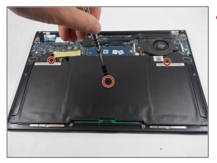
Use a Phillips #00 screwdriver to remove the three 7 mm screws that secure the battery.
