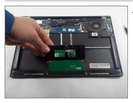
Lift up and pull backwards to remove the touchpad
