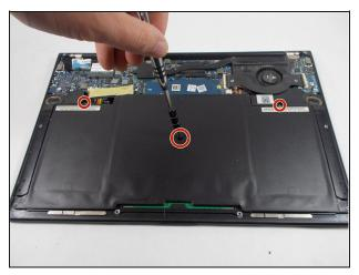
Use a Phillips #00 screwdriver to remove the three 7 mm screws that secure the battery.
