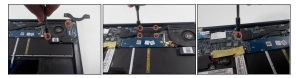
• Use a Phillips #00 screwdriver to remove all seven 6 mm screws that secure the fan and heatsink.
