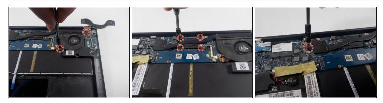
• Use a Phillips #00 screwdriver to remove all seven 6 mm screws that secure the fan and heatsink.
