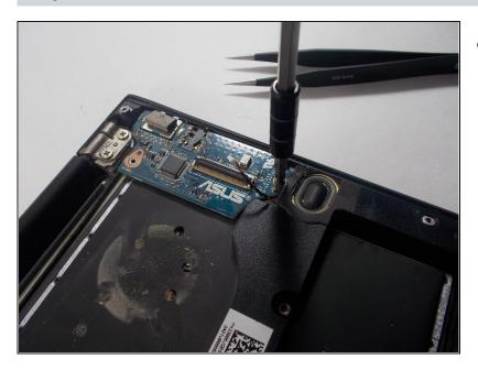
• Use a Phillips #00 screwdriver to remove the 6 mm screw that secures the daughterboard.
