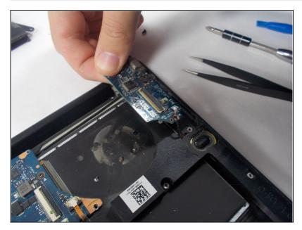
• Remove by carefully lifting the board from the laptop.
