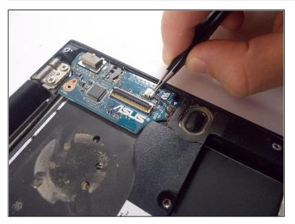
Use tweezers to detach the cable from the board by pulling them gently toward the bottom edge of the board.
