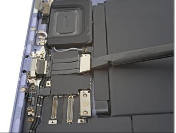
• Use the flat end of a spudger to pry up and disconnect the USB-C port's press connector secured to the frame.
