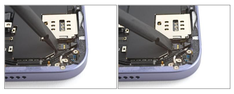
• Use a spudger, an opening tool, or your fingernail to flip up the small, hinged locking flap on the SIM card reader cable's <u>ZIF connector</u>.
