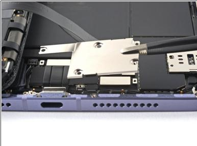
• Use tweezers, or your fingers, to remove the display cable bracket from the frame.
