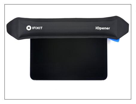
Apply a heated iOpener to the right edge of the device for 90 seconds to loosen the adhesive underneath.
