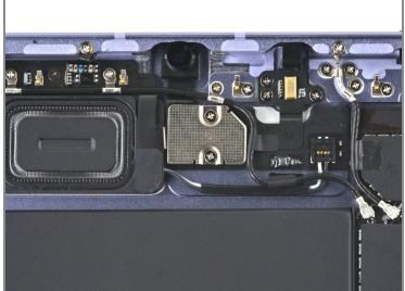
Use a Phillips #000 screwdriver to remove the two 1.2 mm screws securing the front camera shield to the frame.
