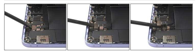
• Use the flat end of a spudger to pry up and disconnect the display cable's two press connectors secured to the frame.
