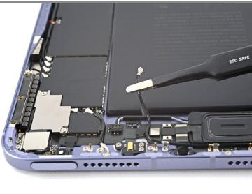
• Use tweezers, or your fingers, to pull the coaxial cable away from the frame, making sure to separate the tape keeping it in place.
