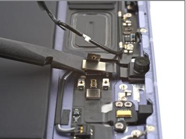
• Use a spudger to pry up and disconnect the front camera board's press connector secured to the frame.
