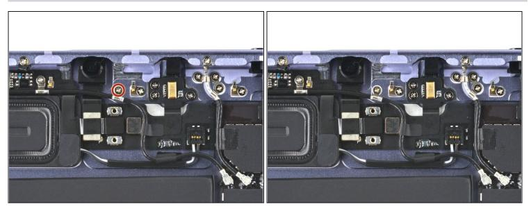
• Use a Phillips #000 screwdriver to remove the 1 mm screw securing the volume button board's coaxial cable to the frame.
