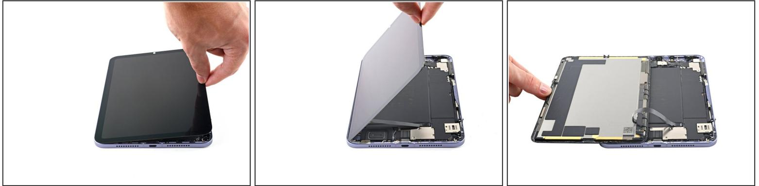
**i** If there's still resistance around the edges of the screen, use an opening pick to cut the adhesive again.
