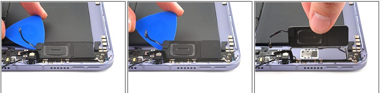
**i** At this point, the perimeter of the speaker should be separated from the frame. If there's still resistance around the edges of the speaker, use an opening pick to cut the adhesive again.
