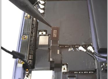
• Use the tip of a spudger to pry up and disconnect the power button board's press connector.
