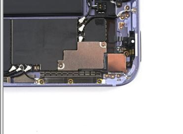
• Use a Phillips #000 screwdriver to remove the two 1.2 mm screws securing the rear camera shield to the frame.
