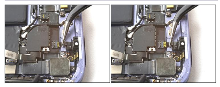
• Use a pair of tweezers to pull the power button board's cable straight out of its ZIF connector on the frame.
