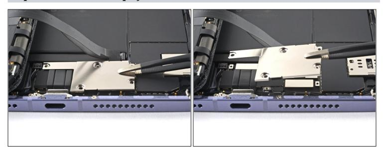
• Use <u>tweezers</u>, or your fingers, to remove the display cable bracket from the frame.
