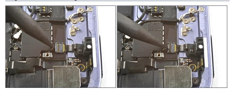
• Use a spudger, an opening tool, or your fingernail to flip up the small, hinged locking flap on the power button board cable's <u>ZIF connector</u>.
