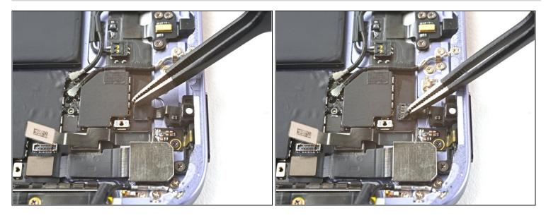
• Use tweezers, or your fingers, to remove the black tape on top of the power button board's ZIF connector.
