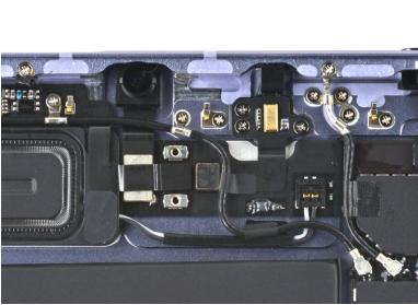
• Use a Phillips #000 screwdriver to remove the 1 mm screw securing the volume button board's coaxial cable to the frame.
