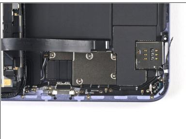
Use a Phillips #000 screwdriver to remove the five 1.2 mm-long screws securing the frame bracket to the frame.
