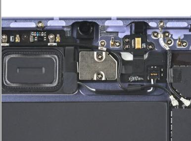
Use a Phillips #000 screwdriver to remove the two 1.2 mm screws securing the front camera shield to the frame.
