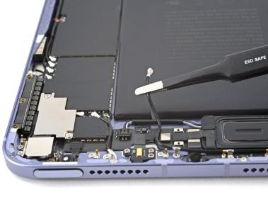
Use tweezers, or your fingers, to pull the coaxial cable away from the frame, making sure to separate the tape keeping it in place.
