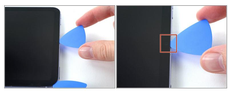
Repeat the heating, slicing, and leaving opening picks for the remaining edges of the device.
