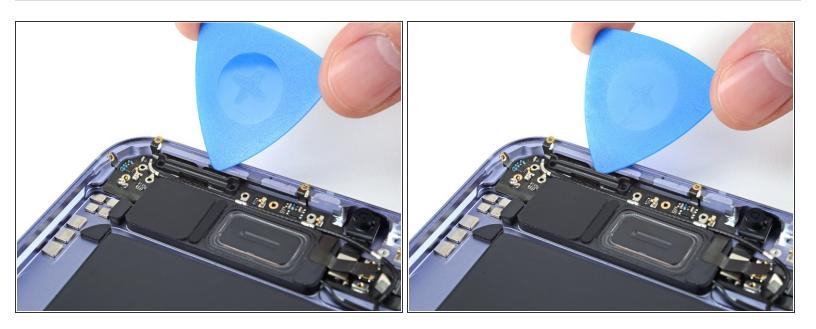
Use an opening pick, or a spudger, to pry the volume button bracket out of its plastic clips.
