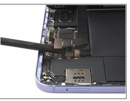
• Use the flat end of a spudger to pry up and disconnect the display cable's two press connectors secured to the frame.
