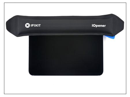
Apply a heated iOpener to the right edge of the device for 90 seconds to loosen the adhesive underneath.
