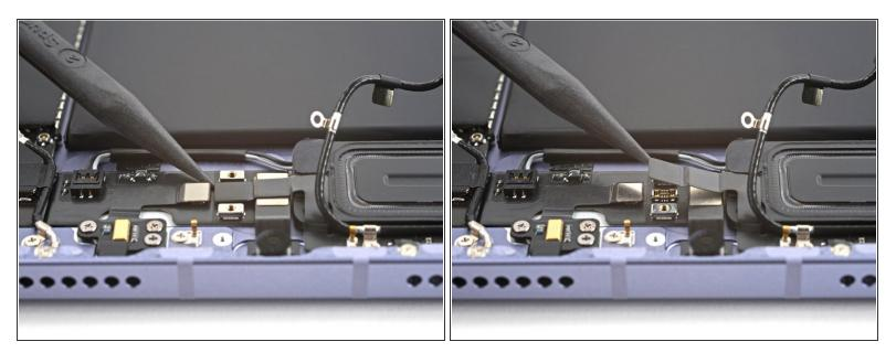
Use a spudger to pry up and disconnect the volume button board's press connector secured to the frame.
