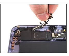
• Gently peel the volume button board away from the frame to completely separate the adhesive.
