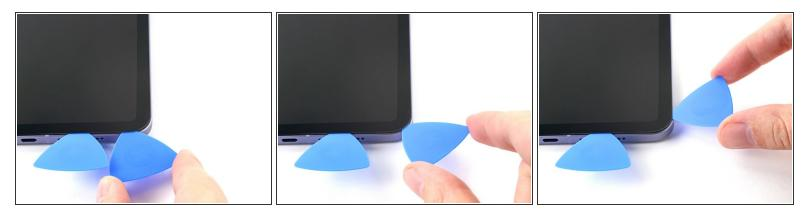
Rotate the opening pick around the bottom-right corner of the device.
