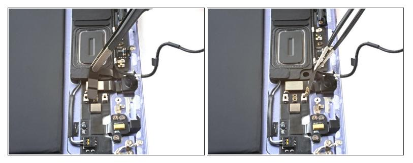
• Use tweezers, or your fingers, to peel back the volume button board's cable from the top speaker.
