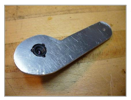
Lens adjustment tool can be used to rotate the lens assembly to adjust or remove the lens.
