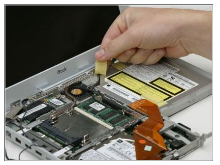
Peel back the yellow tape securing the inverter cable to the optical drive.
