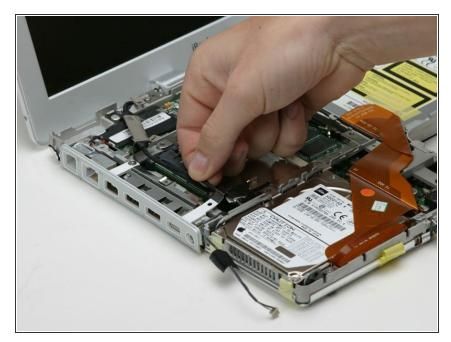
• Deroute the display data and microphone cables.
