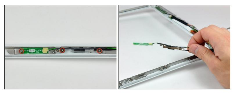
Remove the three Phillips screws securing the reed switch board and the AirPort antenna to the front bezel.
