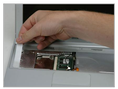
• Peel up the foil tape covering the speaker cable near the ports.
