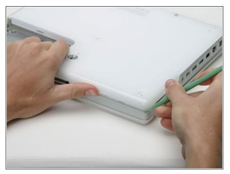
• Continue to run the spudger around the front, right corner. There are two tabs on the port side of the computer, one near the front corner and one near the sound out port.
