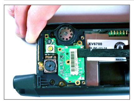
Gently pry off the camera flash circuit board with the spudger.
