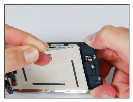
Turn the display assembly over and again carefully insert a metal spudger between the two metal rails along the edge of the display assembly. Gently rotate the spudger to lift the LCD up from the glass.
