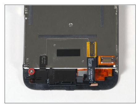
Remove the single Phillips #00 screw from the corner of the display assembly.
