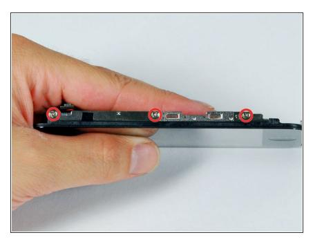
Remove the three Phillips #00 screws from the left side of the display assembly.
