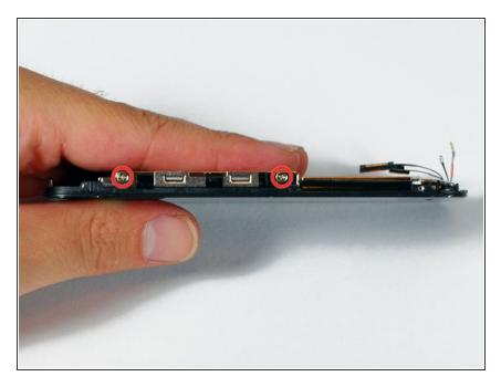
Remove the two Phillips #00 screws from the right side of the display assembly.
