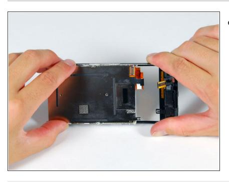
Separate the LCD and glass by sliding the LCD panel away from the ribbon cables on the glass.
