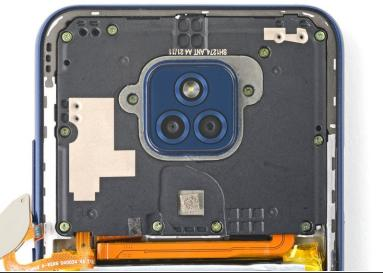
Use your Phillips screwdriver to remove the twelve 3.9 mm-long screws securing the motherboard cover.
