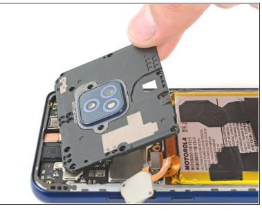
Grab the bottom edge of the motherboard cover and remove it from the frame.
