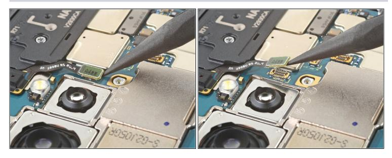
Use the pointed end of your spudger to pry up and disconnect the laser autofocus module press connector.
