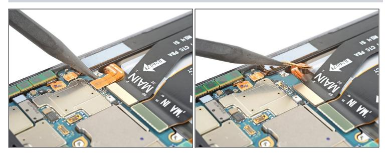
• Use the pointed end of your spudger to pry up and disconnect the battery press connector.
