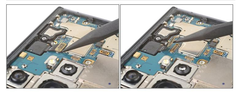
Use the pointed end of your spudger to pry up and disconnect the front-facing camera press connector.
