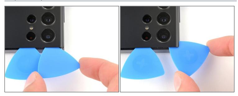
$\triangle$  Only insert the pick up to 4 mm, as you may damage the cameras.
