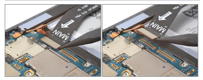
• Use the pointed end of your spudger to pry up and disconnect the screen press connector.
