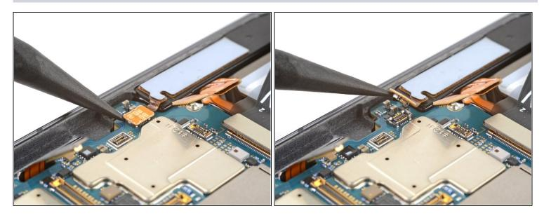
• Use the pointed end of your spudger to pry up and disconnect the stylus' press connector.
