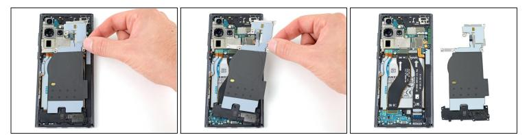
Grab and remove the NFC, wireless charging coil, and loudspeaker from the frame.
