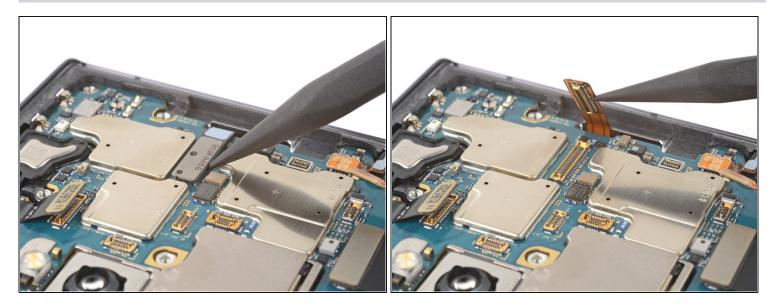
• Use the pointed end of your spudger to pry up and disconnect the fingerprint reader press connector.
