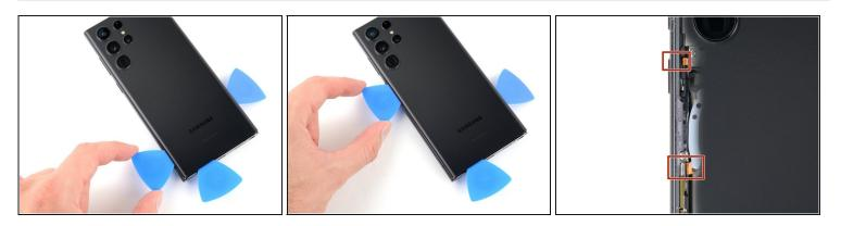
• Slide your opening pick along the left edge to slice the adhesive, stopping when you reach the power button.
