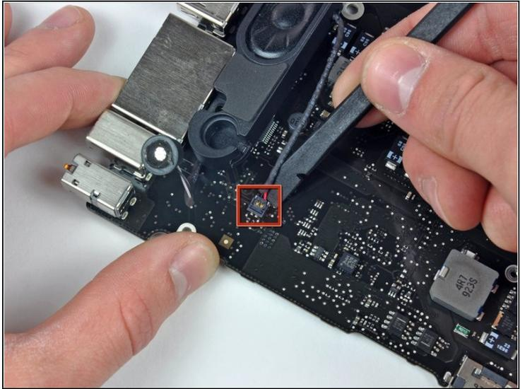
ⓘ If necessary, peel up the tape covering the left speaker connector.
