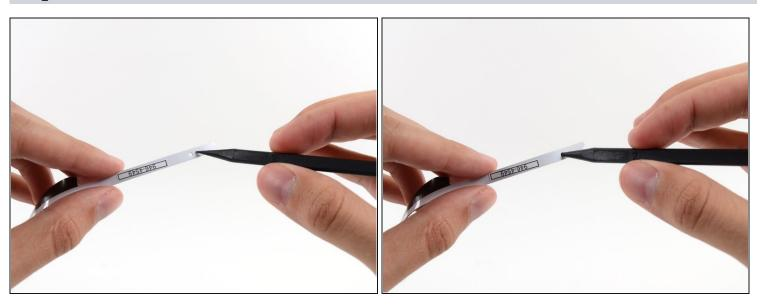
Insert the tip of a spudger into the hole at the top of the strip from the side that still has a backing on it.
