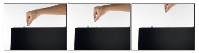
• Remove one side of the protective film from Strip 11 by pulling its tab straight up.
