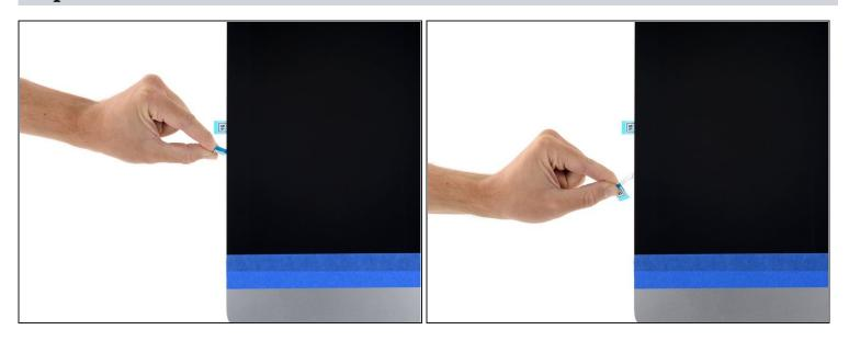
• Repeat the previous steps to remove the protective films from all the remaining adhesive strips (labeled 11, 12, and 13).
