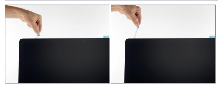
• Remove the other side of the protective film from strip 11.
