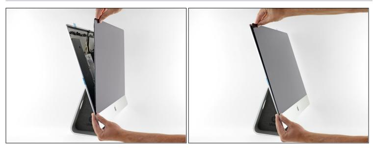
• Gently lay the display in place over the iMac, and align it carefully.
