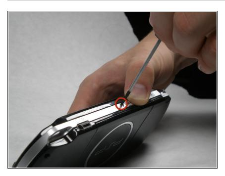
Then, remove the single screw from the bottom edge of the PSP (which is positioned next to the barcode).
