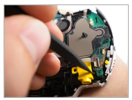
Carefully bend back the black tab holding the power jack in place and start pulling the jack up to release it from this clip.
