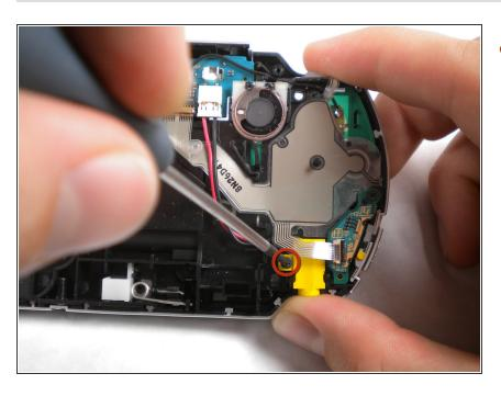
Remove the screw from the power jack.
