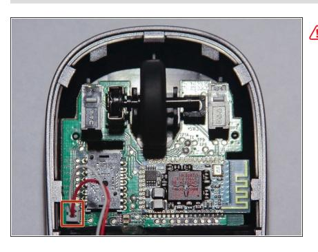
Use the appropriate tool to remove gently the power connector. Don't use your finger, you might brake the cable
