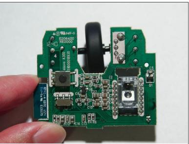
The micro switch can be replaced by OMRON D2FC-F-7N but you need to trim the solder terminals with a flush wire cutter
