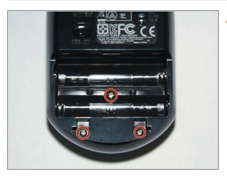
3 Phillips screws are located under the battery cover, unscrew them
