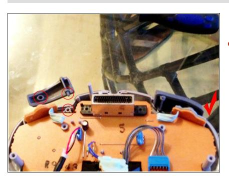
Reinsert the buttons, ensuring that the rubber, cylindrical pieces protruding from the buttons are lined up with their corresponding circuits. Follow these steps in reverse order to reassemble your device.
