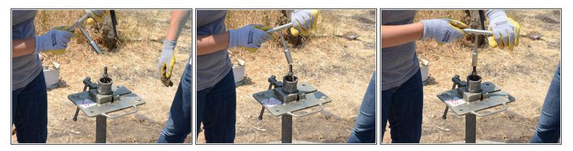
• Reattach the T-handle to the top of the pump rod.
