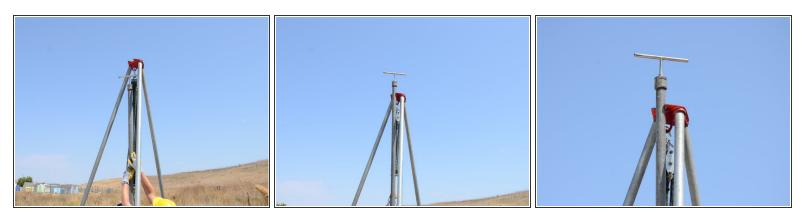
(i) The tripod has an indentation built into its top to guide the riser pipe.
