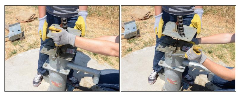
• Tighten the rod clamp against the pump rod.
