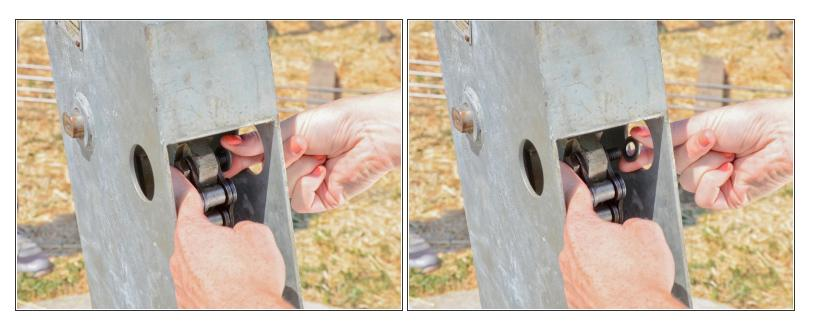
• Remove the washer from the chain bolt.
