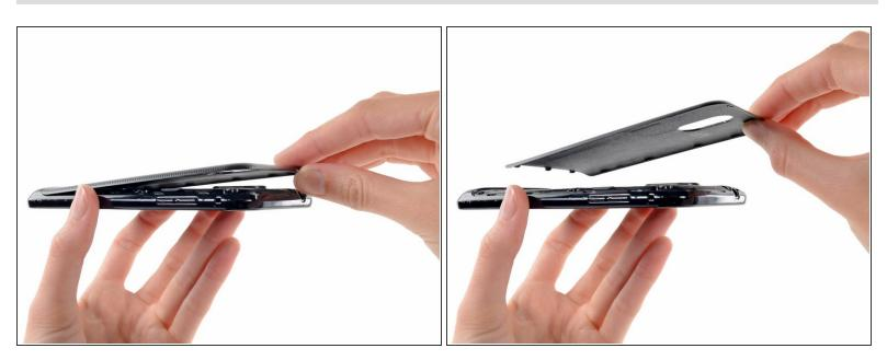
Lift and remove the rear case.
